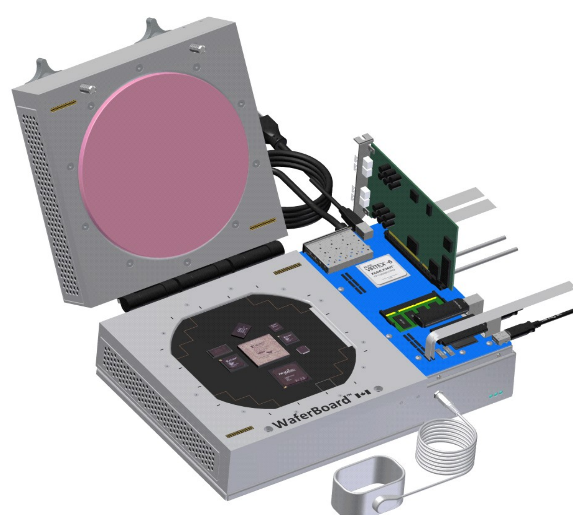
Figure 1: A 3-D model of the WaferBoard™: the black surface is a 200mm wafer, covered by more than a million programmable I/Os. They are capable of sensing the position of user ICs, driving current and propagating digital signals.
