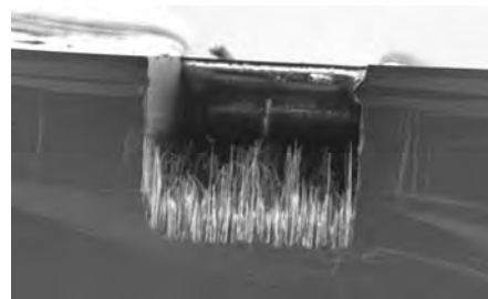
Figure 7: SEM Image showing black silicon issue
