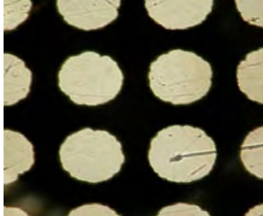
Figure 1: Optical image of backside illuminated TSVs: 200µm diameter-600µm thick wafer
